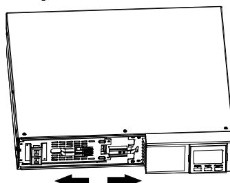
Disconnect battery wires.
