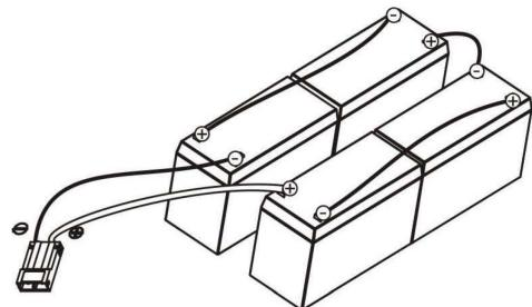
Step 3: Put assembled battery packs on one side of plastic shells.
