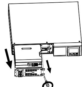
Pull out the battery box by removing two screws on the front panel.
